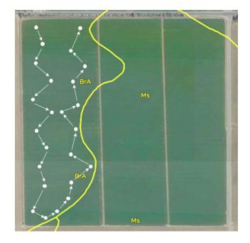
**Figure 1:** Soil sampling plan for a representative sample from a field or management area. The Picture is a screenshot of a field from Google map using the SoilWeb application.
